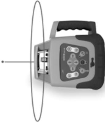
The PLS HVR 505 has third leveling axis (z-axis). Place the instrument as shown. The plumb beam will be leveled automatically. The turning rotor head projects an upright plane to the plumb beam at an angle of  $90^\circ$ . To adjust the alignment line use the arrow keys to move the laser beam right and left.
