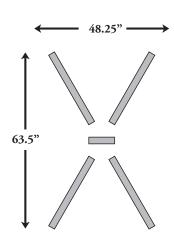
For maximum wind resistance: All four (4) legs must be fully telescoped and in the down and locked position when using either 36"x36" or 48"x48" roll-up signs
