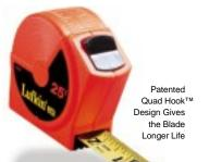
The weakest point of any measuring tape is the center of the blade's concave surface. The end hook on all power tapes have historically been riveted through this point increasing the potential of blade or end hook failure. Through extensive engineering, research and testing, Lufkin has developed the Quad Hook.
