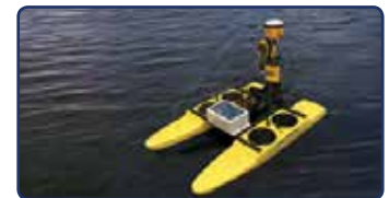
HyDrone™ ASV with Trimble SPS 585 and TSC3
