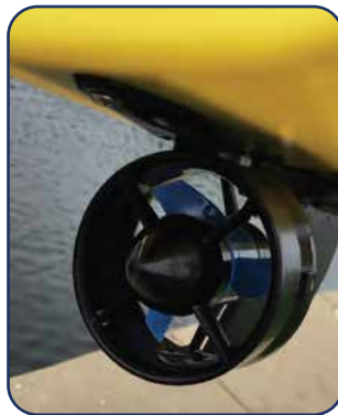
Power differential thrusters for maneuverability
