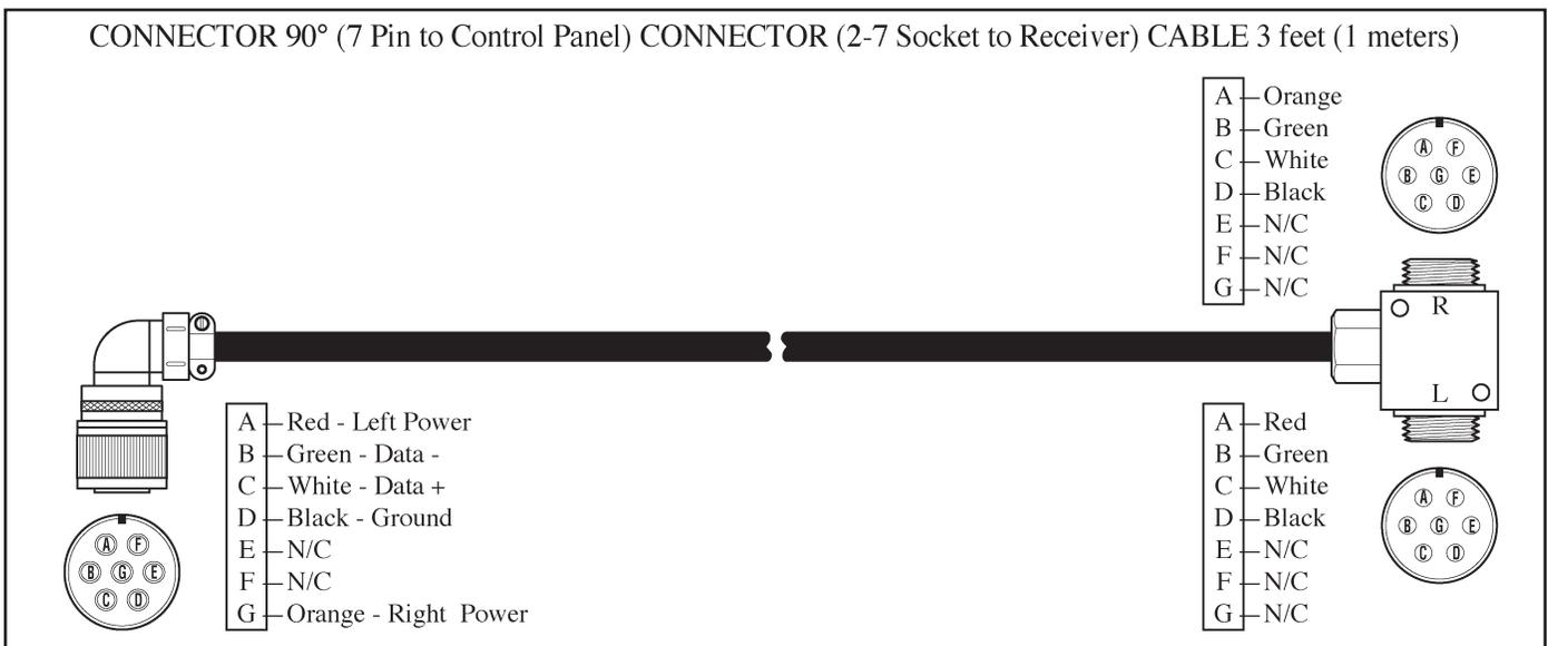
Figure 17. Receiver Junction Cable
