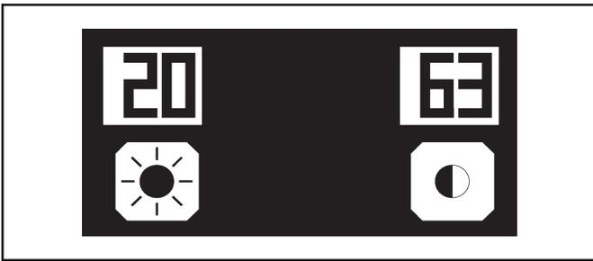
Figure 8. LCD Brightness and Contrast Edit Mode
