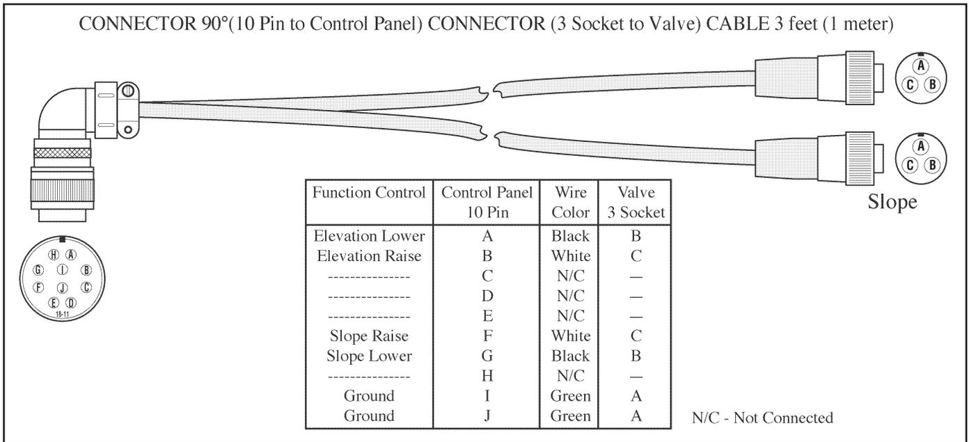
Figure 19. Valve Cable
