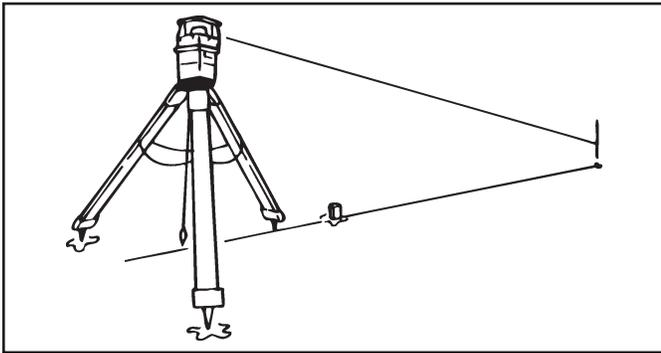
Figure 25. Method One: Align Rotating Laser with Grade Stakes
