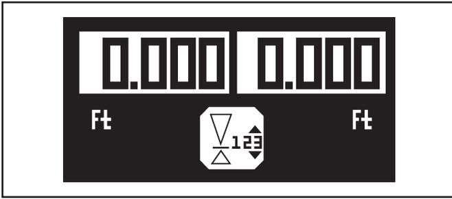
Figure 11. Reference Elevation Edit Mode
