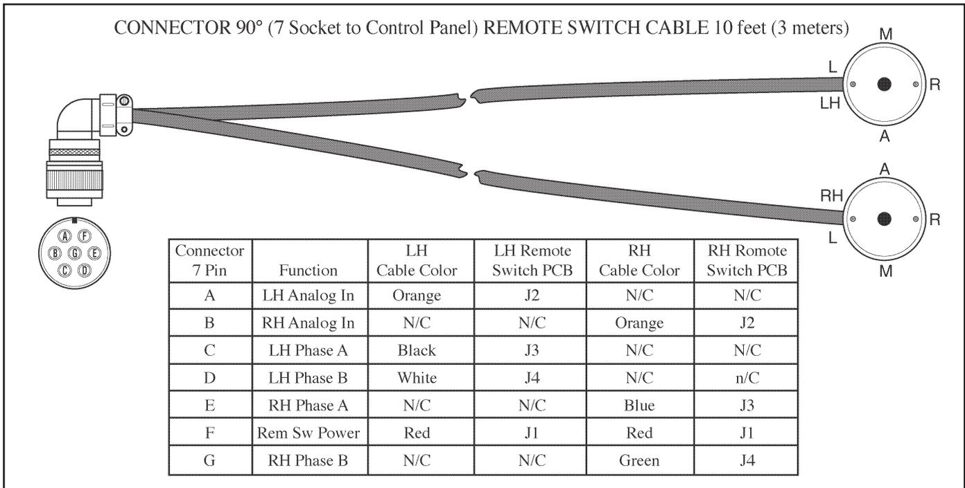
Figure 20. Remote Switches Cable
