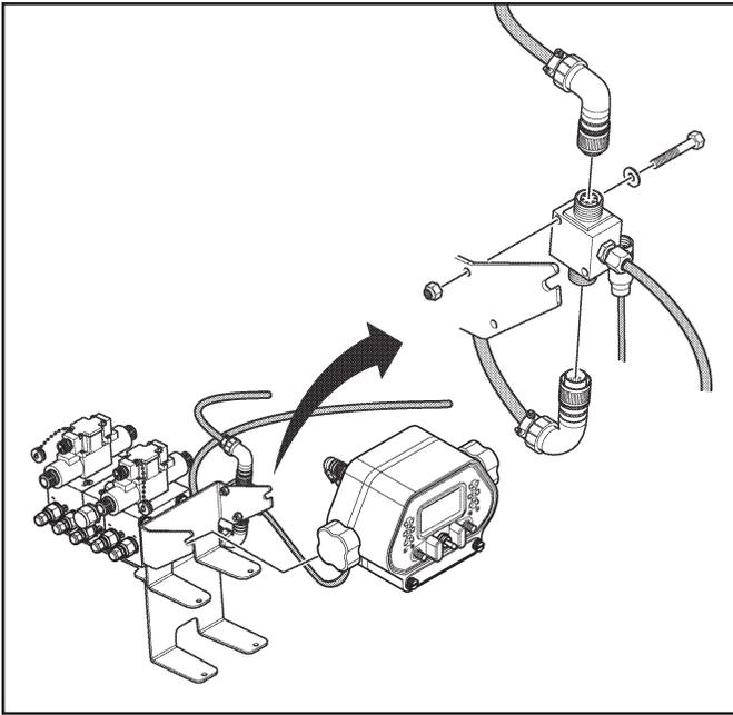
Figure 24. Junction Block and Laser Receiver Cables
